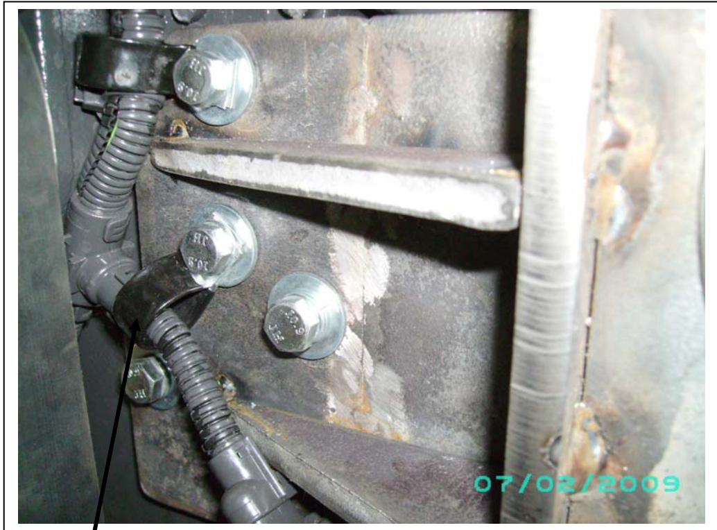
Four front M8 mount bolts.
